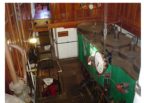
A triple-expansion marine steam engine on the 1907 oceangoing tug Hercules
