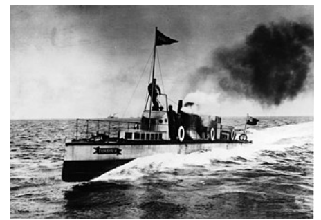
Turbinia – the first steam turbine-powered ship
