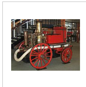
British horse-drawn fire engine with steam-powered water pump
