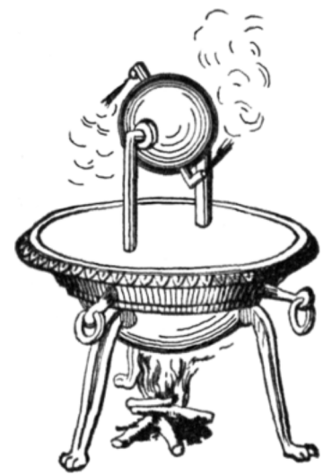
An aeolipile rotates due to the steam escaping from the arms. No practical use was made of this effect.
