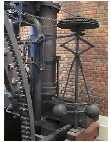
Centrifugal governor in the Boulton & Watt engine 1788 Lap Engine.
