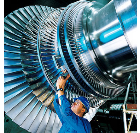
A rotor of a modern steam turbine , used in a power plant
