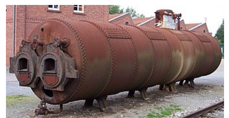
An industrial boiler used for a stationary steam engine
