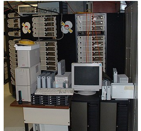
The Borg, a 52-node Beowulf cluster used by the McGill University pulsar group to search for pulsations from binary pulsars
