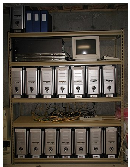
A home-built Beowulf cluster composed of white box PCs
